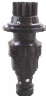
■ SLEWING UNIT GEAR
